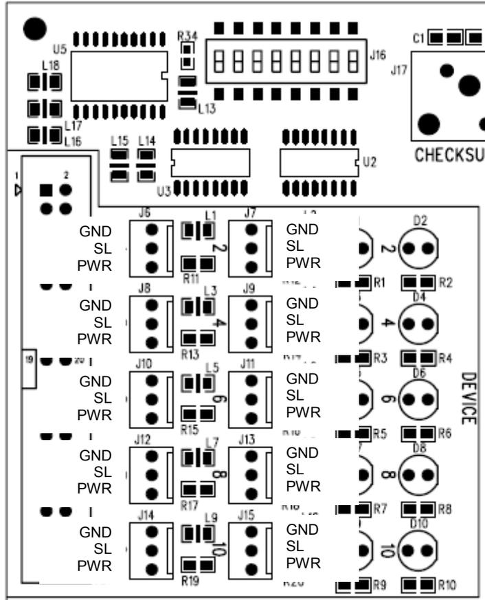
Diagram 3.2 Pin assignments for each connector 'J1' - 'J10'
