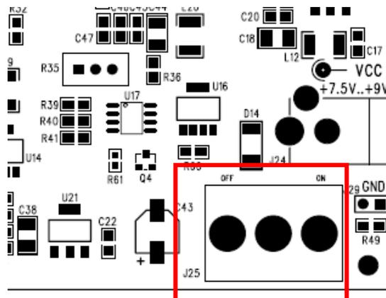
Diagram 2.3 On/Off position of power switch
