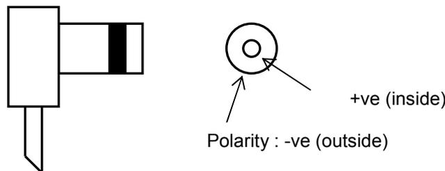
Diagram 2.2 Polarity of DC Jack
