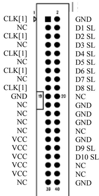
Diagram 3.3 Connection between 'J21' and devices
