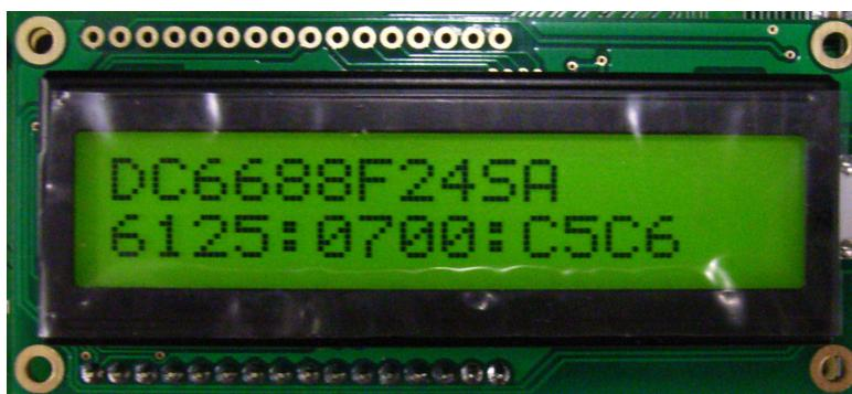
Diagram 4.1 Device name in the 1<sup>st</sup> line and Model:Version:Checksum in the 2<sup>nd</sup> line
