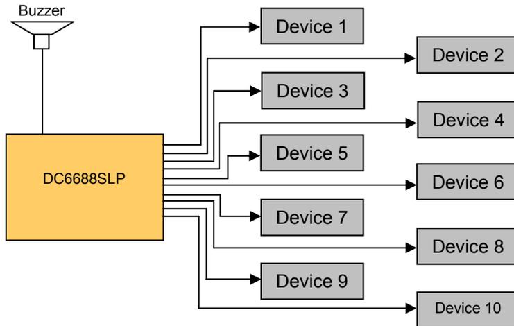
Diagram 3.1 Connection between SL Programmer board and device
