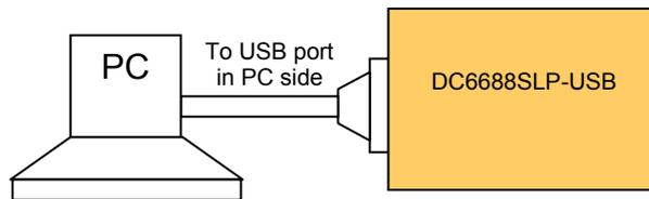
Diagram 2.1 Connection between SL Programmer board and PC
