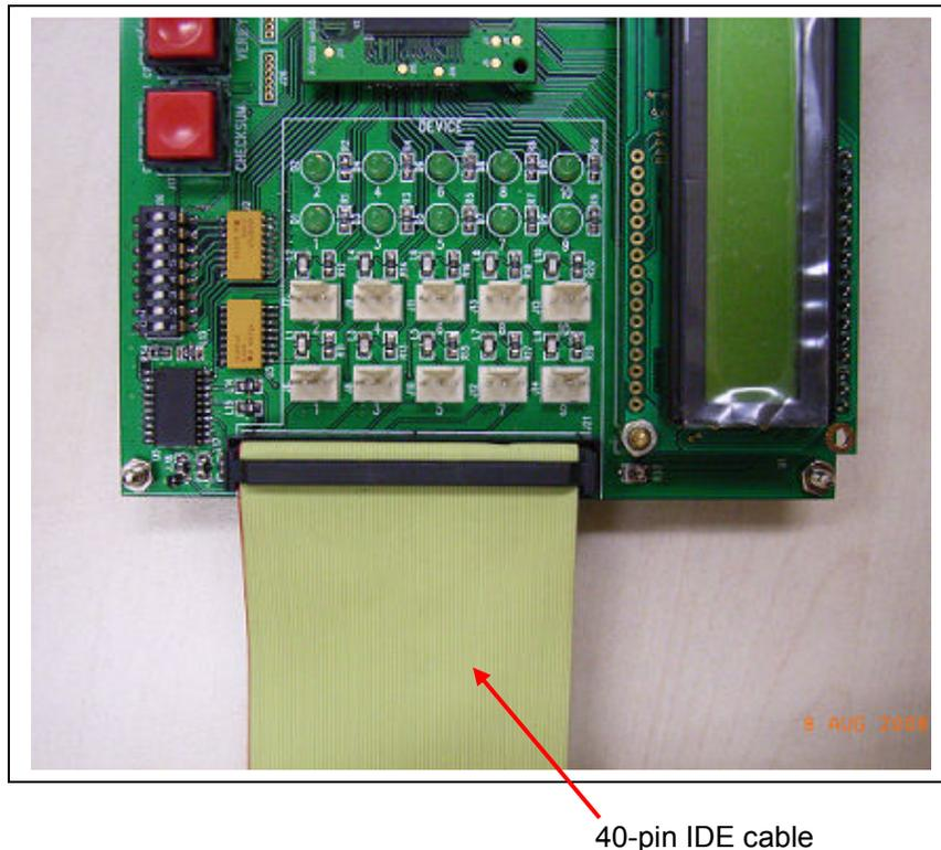
Diagram 3.4 IDE cable on the connector
